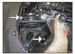
14. Install the heat shield assembly onto the inner fender; secure the mounting bracket to the factory airbox mounting location with the provided hardware. The inserted nut is to be placed in the hole of the inner fender and then secured by tightening the assembly's bolt.
