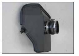
13. Install the silicone hump hose (084057) onto the filter adapter and secure with the provided hose clamp.
