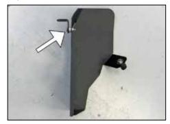
9. Install the heat shield mounting bracket (070066) onto the heat shield as shown using the provided hardware and spacer.
