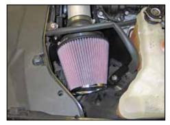
25. Install the K&N<sup>®</sup> air filter and secure with the provided hose clamp.
