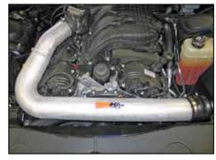
19. Install the K&N<sup>®</sup> intake tube into the silicone hump hose and then into the silicone hose on the throttle body.
